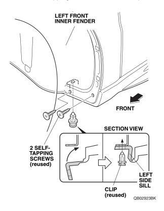
20. Secure the rear of the left side sill with the two self-tapping screws removed in step 3.
