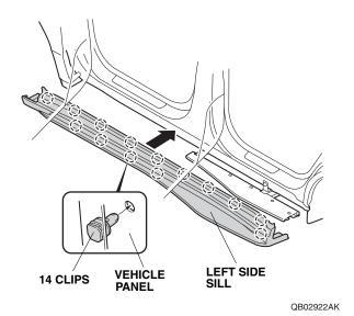
18. Secure the front of the left side sill with the one clip removed in step 2.
